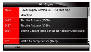
Figure 4-12 Sample Display DTC Screen
