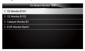
Figure 5-29 Sample CAN vehicle test screen
