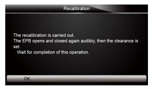
Figure 4-76 Sample Recalibration Operation Screen
